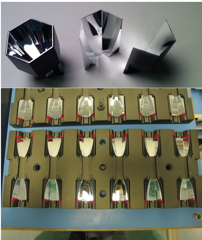
Fig. 10 Top: A picture of an assembled cone (left) and of the two halves before being glued together. Bottom: photo of the jig used to glue 24 half-cones together.
