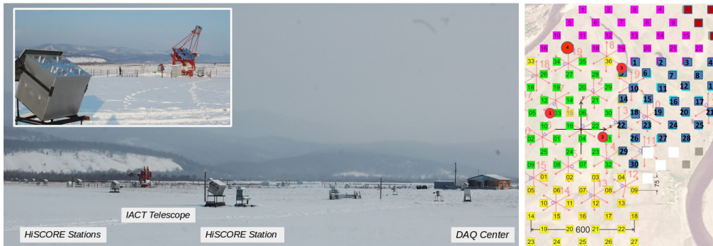
Fig. 1. Overview of the TAIGA Observatory. Left: Panoramic view with the array of TAIGA-HiSCORE stations and IACTs, and the DAQ-center. By early 2020, 1 km 2 of HiSCORE and three IACTs will be installed. Insert: a HiSCORE station and the IACT. Right: Schematic view of the HiSCORE array (~100 stations, grouped in 4 color-indicated cluster) and the TAIGA-IACTs (red dots "1,2,3") and the new TAIGA-SST-1M location (red dot "4").
